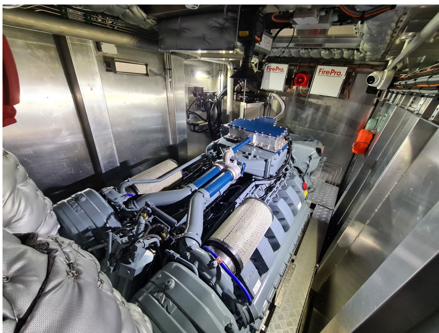
Compact diesel engine for dual fuel operation. The MAN D2862 LE448 – 749 kW (1029 hp) at 2100 rpm.
