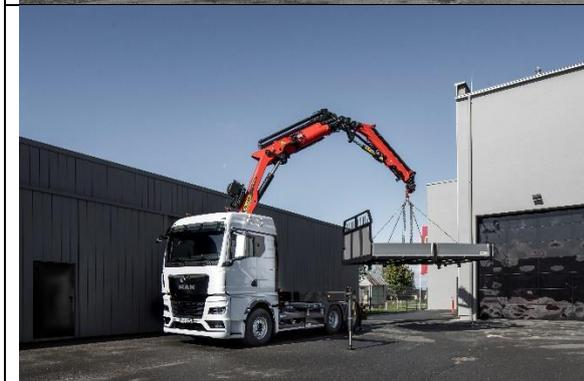
Large loading cranes with a long reach lift heavy loads. MAN offers chassis designs with industry-specific features such as the MAN TGX 33.510 6x4 with 10-ton front axle.
