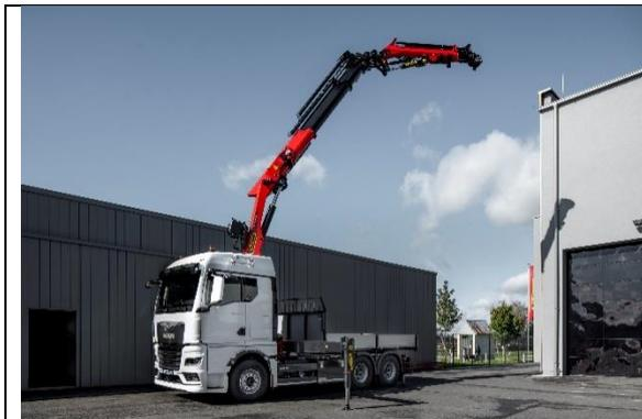
The MAN TGX 33.510 6x4 with GM cab has been fitted with a heavy duty loading crane with four supports by the body manufacturer; on the front of the crane and at the rear directly on the frame behind the rear axles.
