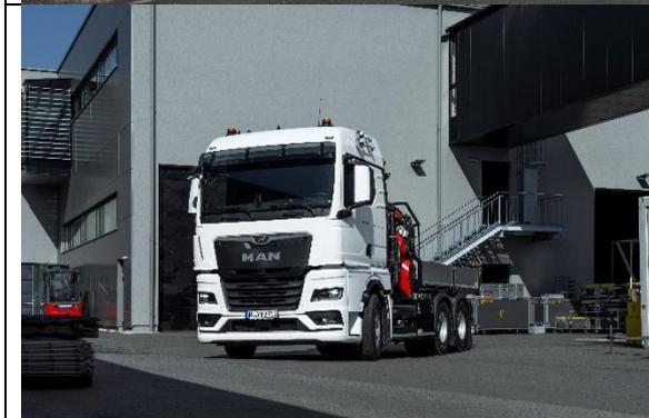
In driving position, the heavy duty loading crane on the MAN TGX 33.510 6x4 is inconspicuous. The lifting accessories and crane attachments can be transported within easy reach in the loading area.
