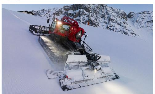
The MAN D3876 for the PistenBully 800 has also been modified for cold start capability, use up to 2,500 metres in altitude without power reduction and extreme lean angles.
