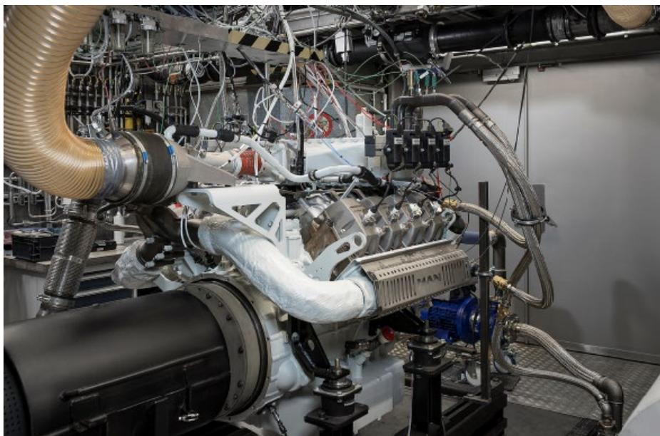
*MAN Engines is currently testing a stationary combustion engine for combined heat and power generation for operation with hydrogen on its test bench.*
